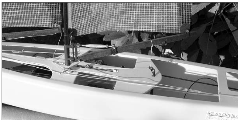
Details of the prototype: The deck openings are covered with an adhesive foil during sailing. The mast fittings are adopted from Graupner's racing Micro Magic. Photo by ©Arne Semken.
