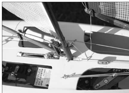
The keel and the mast can be moved by 10 mm to get the right trim for different weather conditions. Photo by ©Arne Semken.
